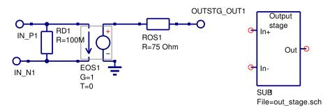
Figure 11: Modular macromodel output stage.
