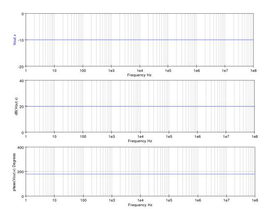
Figure 2: Gain and phase curves for a basic OP AMP inverting amplifier.
