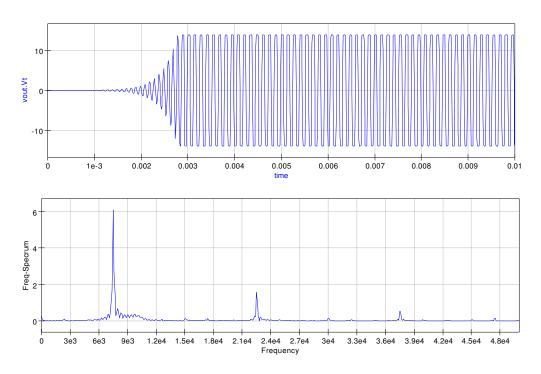
Figure 36: Simulation waveforms for the circuit shown in Fig. 34: OP27 AC + slew rate + vlimit macromodel.
