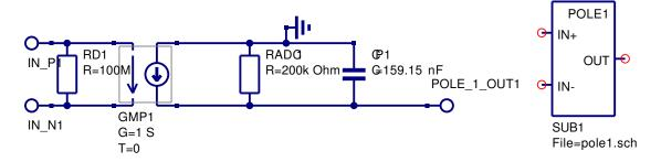
Figure 9: Modular OP AMP first voltage gain stage.
