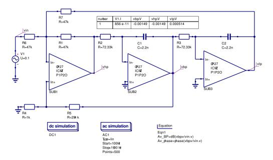
Figure 31: Three OP AMP state variable filter.
