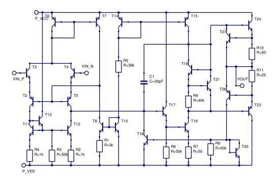
Figure 3: Transistor level circuit for the UA741 operational amplifier.
