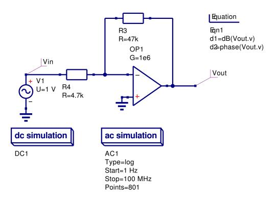
Figure 1: Ques schematic for a basic OP AMP inverting amplifier:Ques OP AMP has G=1e6 and Umax=15V.
