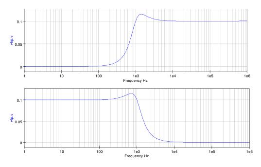
Figure 33: State variable low pass and high pass response for Q = 1,  $R5 = 2k\Omega$ .
