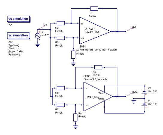
Figure 20: Simulation of OP AMP common-mode performance.
