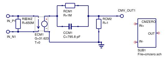
Figure 18: Common-mode zero macromodel
