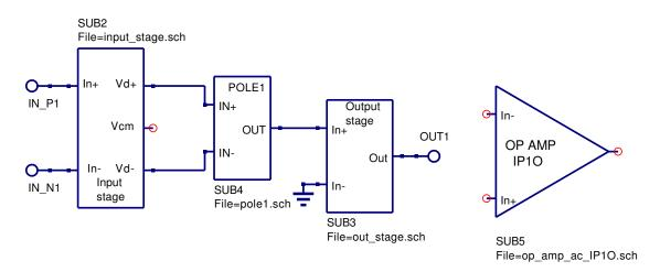
Figure 12: Simple AC OP AMP macromodel.
