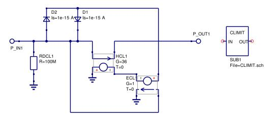
Figure 28: OP AMP output current limiter macromodel.
