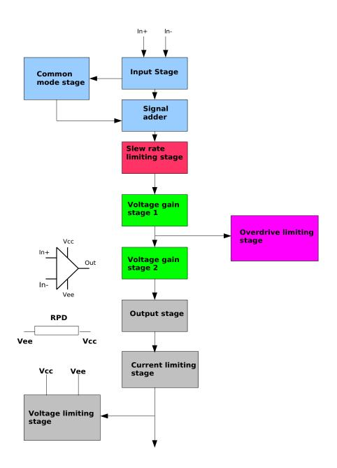
Figure 7: Block diagram of an operational amplifier macromodel.
