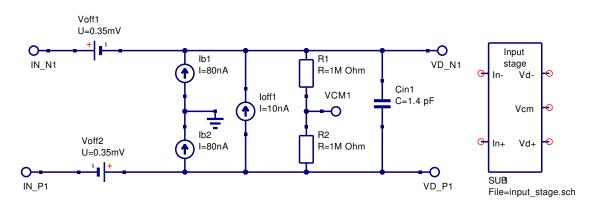
Figure 8: Modular OP AMP input stage block.
