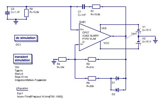
Figure 37: Wien bridge oscillator with automatic gain control.
