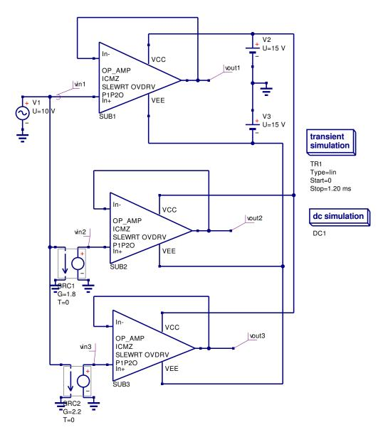
Figure 26: OP AMP overdrive and output voltage limiting test circuit.
