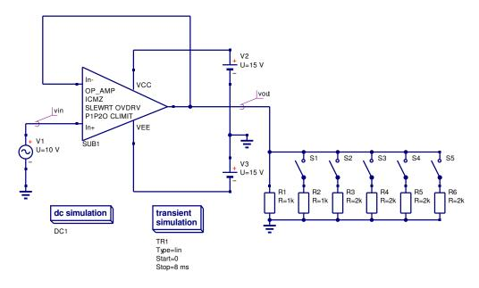
Figure 29: OP AMP output current limiter test circuit.
