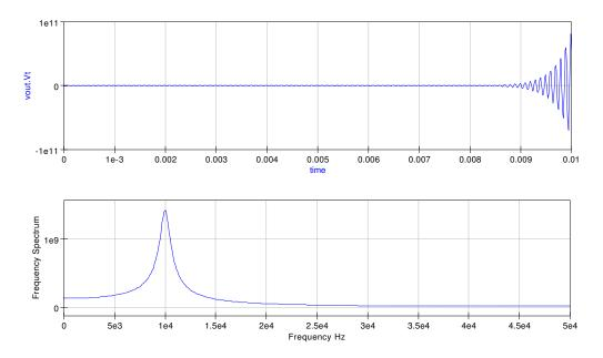
Figure 35: Simulation waveforms for the circuit shown in Fig. 34: OP27 AC macromodel.
