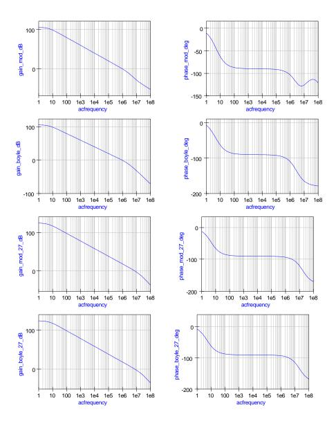
Figure 48: Open loop voltage gain simulation waveforms for the modular and Boyle UA741 and OP27 macromodels.
