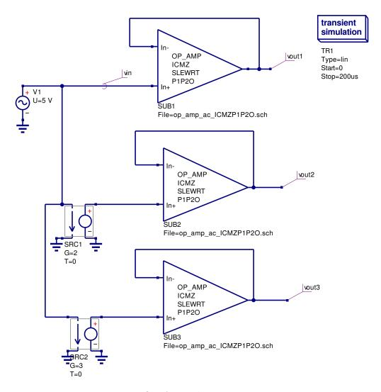
Figure 23: OP AMP slew rate test circuit.
