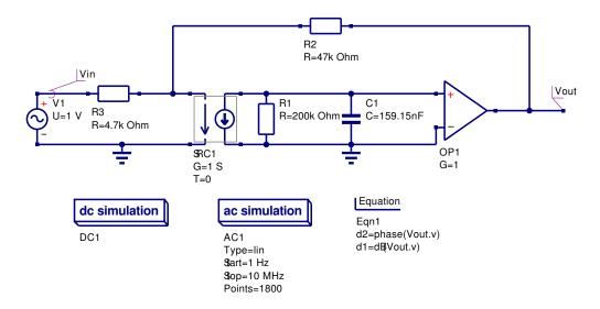
Figure 5: Modified Ques OP AMP model to include single pole frequency response.
