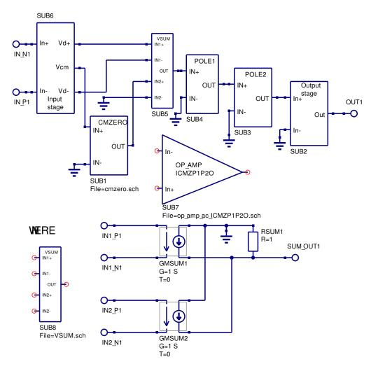
Figure 19: AC macromodel including common-mode zero.
